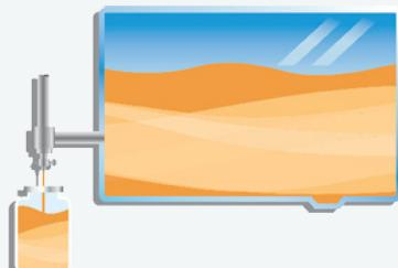
A permanent sampling port provides a consistently accurate sample collection source and is applicable to both pressurized and non-pressurized systems.
