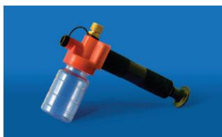
A petcock valve or similar sampling device is permanently installed upstream of any filters. A vacuum pump draws fluid through tubing and into the sample jar.
