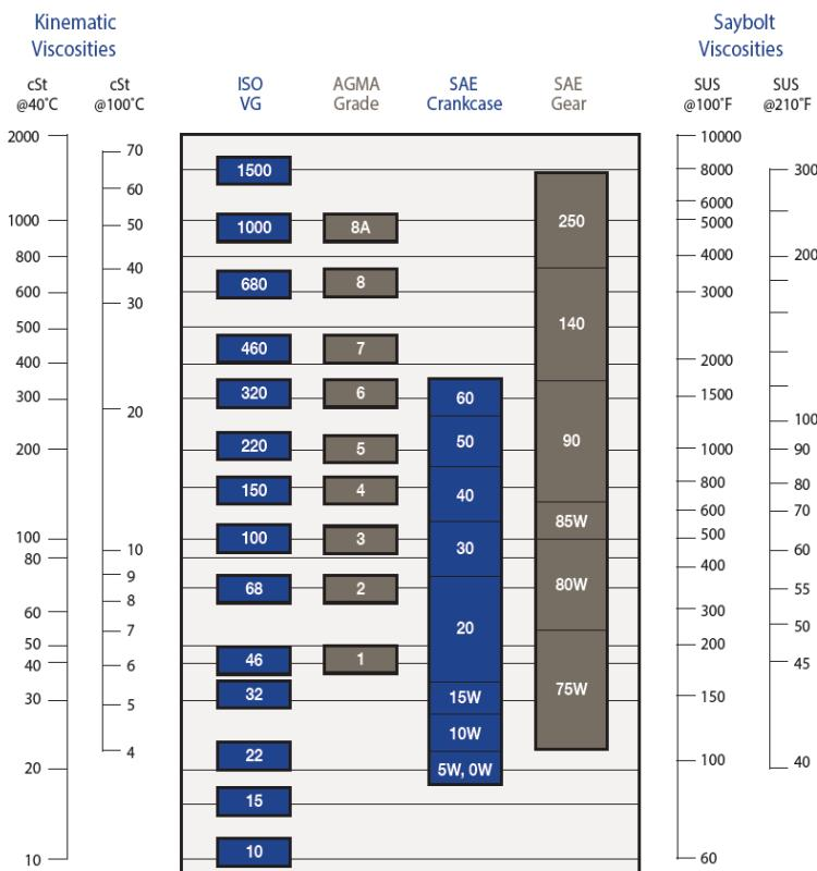
\* This grade comparison is a general guide that applies to viscosity at several different reference temperatures but does not evaluate total lubricant quality. These comparisons are based on a 95 VI product.
